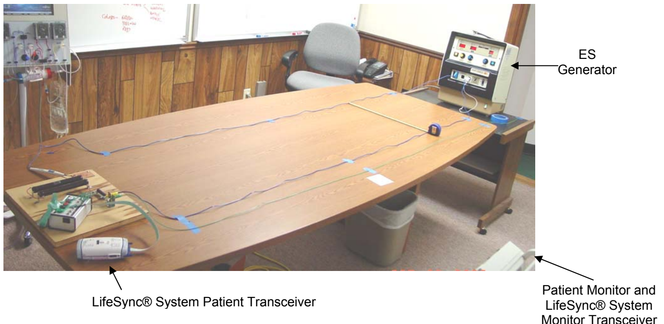
Figure 3 - LifeSync® System ESIS Test Setup
