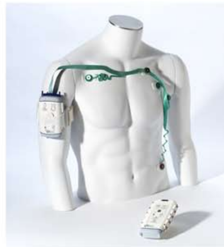
The LifeSync Wireless ECG System by GMP Wireless Medicine Inc. uses Bluetooth technology to eliminate lead wires and trunk cables. It works with existing hospital equipment.
